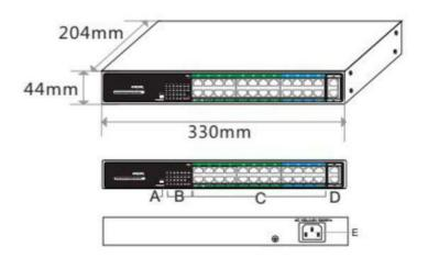
A.Multi-functional switch B.Working LED indicator
