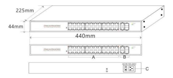
A.24\*PoE Ports B. 2\*Sets Combo Ports C.100-240VAC,50/60Hz
